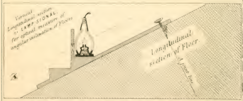
Special forms of apparatus, employed in measuring in the Grand Gallery.
