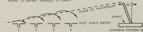
D EXCITATION OF PROGRESSIVELY DIFFERENT PHASES CAUSES WAVEFRONT TO DEPART AT AN ANGLE TO ARRAY
