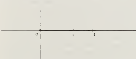
Vector Representation of Current and Voltage in a Resistive Circuit
