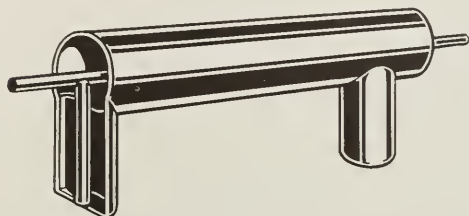
Rigid Coaxial Cable with Metallic Insulators
