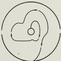
Path of an Electron Delivering Energy to the Alternating Field
