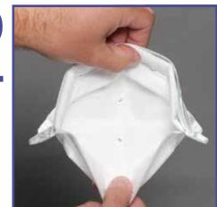
Unfold the respirator by pulling top part (with nosepiece) up and bottom part down so the respirator is open all the way. Straps should be held on the top panel.
